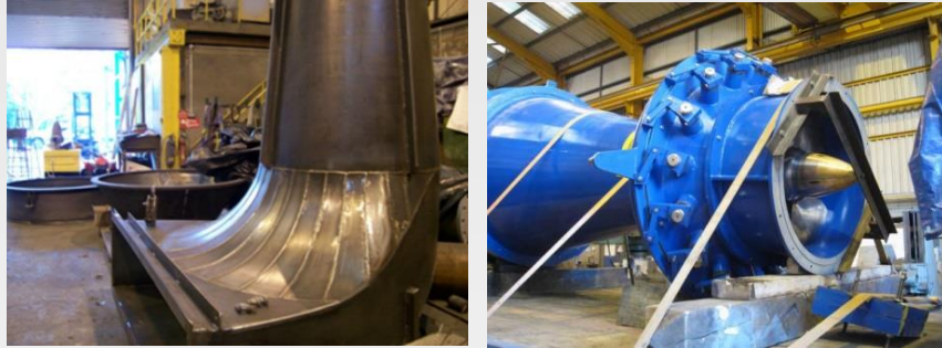
Low Head Kaplan Turbine and Draft Tube
