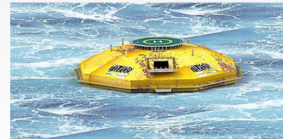
TALOS Wave Energy Converter Multi-Axis, Omni-Directional Point Absorber Style WEC completely enclosed with internal inertial mass using Hydraulic Cylinders or Linear Generators PTO
